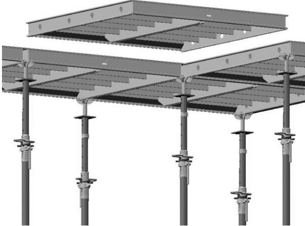
1. Insert panels into the DeckFast Bearing Supports from above the bearing supports.
